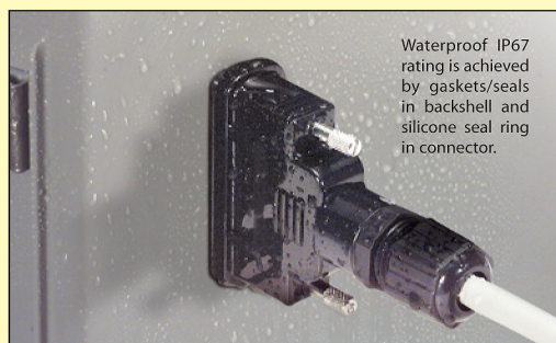
Mate connectors and secure backshell thumbscrews to threaded jackscrews.
